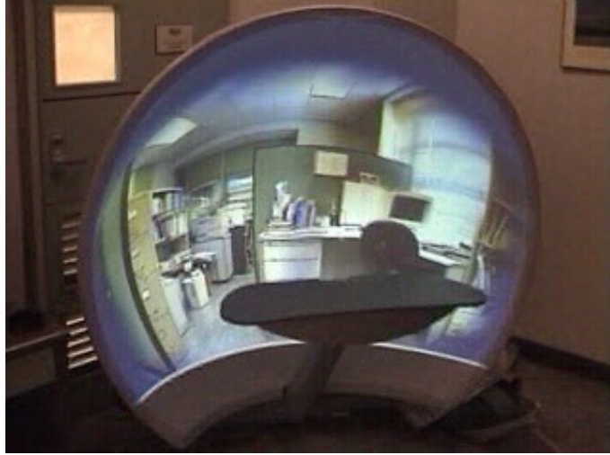
Fig. 11. Panoramic display of indoor scene on the hemispherical screen.
