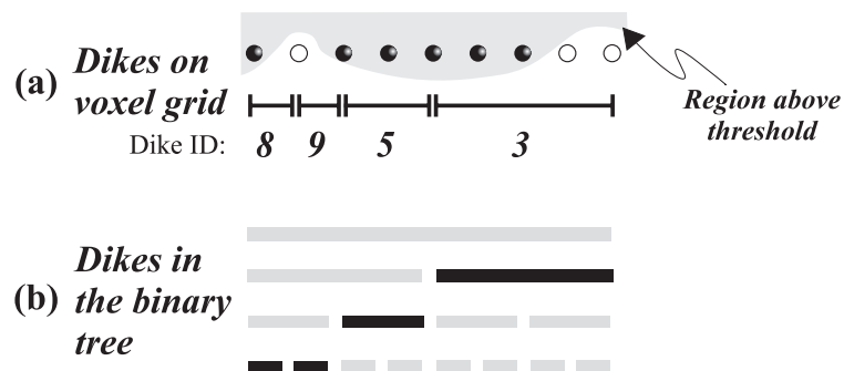
Figure 3-5: (a): The lign is subdivided into length-maximal dikes by algorithm InitSimple . (b): The dikes visited when walking through the lign.
