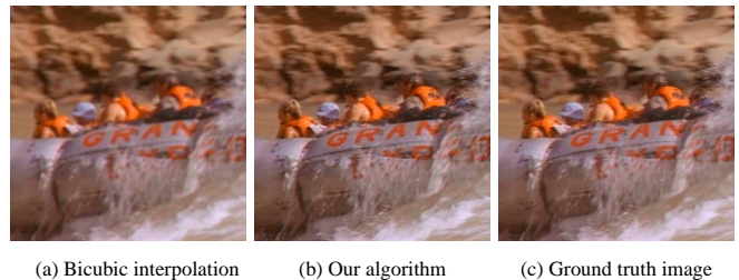
Figure 6: Comparison with the ground truth image. The peak signal-to-noise ratio (PSNR) values for bicubic interpolation and our algorithm are 37.78 dB and 38.81 dB, respectively.
