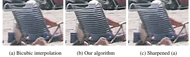
Figure 5: Comparison with bicubic interpolation. In this experiment, we magnify the target frame of Beach two times in both dimensions using bicubic interpolation (a) and our algorithm (b). The result by bicubic interpolation is blocky and blurry. With sharpening (c), errors are exaggerated. Our algorithm generates image with better quality.
