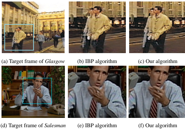
Figure 7: Comparison with IBP algorithm. Image (a) is the target frame from Glasgow video and image (d) is from Salesman sequence. Both clips are in QCIF resolution ( 176 \times 144 ). We magnify the images two times using IBP ((b)&(e)) and our algorithm ((c)&(f)). Parts of the super-resolved images are blown up for clarity. Images by IBP exhibit apparent errors at the left-most person in (b) and at the hand in (e).
